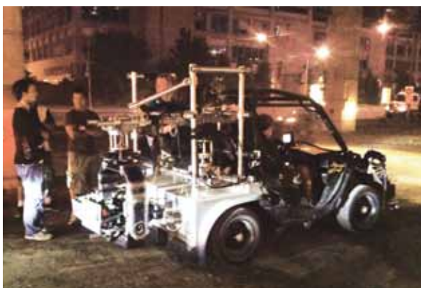
WFW Specialty vehicle " Commander " with Stabilized Scorpio head on the set of " The Transporter " TV series.
