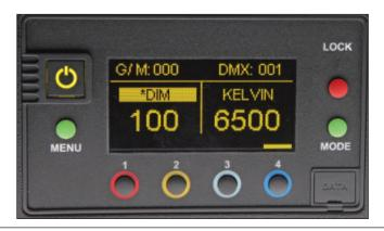
The default setting for **DIM** is that smoothing is on. When smoothing is on, it introduces a time lag such that the individual dimming steps are less noticeable. However, when working in DMX and instant response is required, it is recommended that smoothing be turned off. The **\*DIM** designates that the smoothing function is off.
