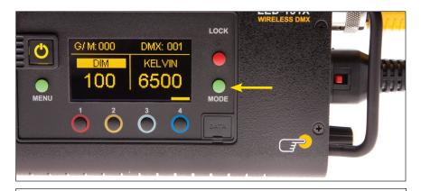
Press the Mode button to select **Dim**. Rotating the control knob will dim the light of the fixture. Default setting is Fine. Press the Control knob to toggle between **Fine** and **Coarse** increments or when selecting options within menus. When the power is turned off or removed, the display will remember its last setting.
