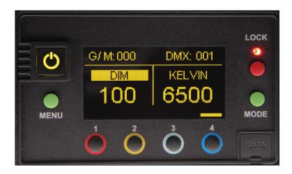
Press the **Lock** button to lock the Dim, Kelvin and G/M setting (Applies to White, Gels/Hue, RGB or FX Modes). A red indicator light will display in Lock mode. Manual controls will be disabled. To unlock, press the Lock button again. The red indicator will turn off.
