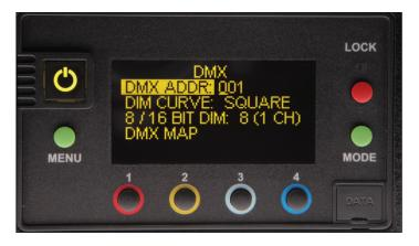
Press the Menu button to select **DMX**. Press and turn the control knob to select individual digit settings for a valid address from 1-512. On the main display, "**X**" next to DMX indicates DMX signal is present.
