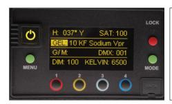
In **Gels/Hue** mode (in addition to **G/M** control), **Gel, Hue** angle and **Saturation** adjustments are available. Kino Flo Presets and industry standard preset Gels are included. Press Menu, select General and press control knob to change Mode to Gels/Hue.
