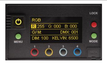
In **RGB Color** mode (in addition to G/M control), individual RGB (Red, Green, Blue) adjustments are available. Press Menu, select General and press control knob to change Mode to RGB.
