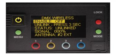
The LED Controller/Fixtures include a built-in Lumen Radio receiver and can be operated wirelessly with a Lumen Radio transmitter (sold separately). For more information on Lumen Radio Receiver/Transmitter, see www.LumenRadio.com.
