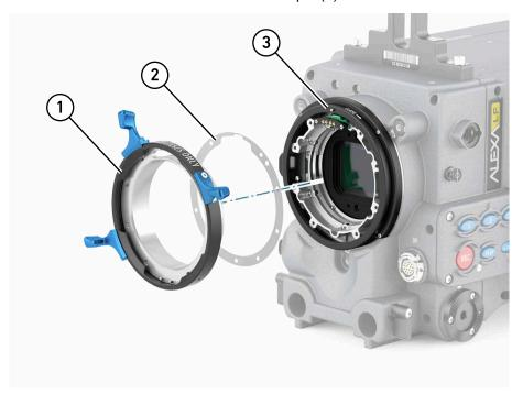
9. Fasten the lens lock, still in position OPEN (2), back to the LPL mount; use four of the eight torx screws (1) hand-tight:
