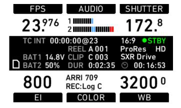
The HOME screen is the ALEXA's default screen. It shows the most important camera parameters and gives quick access to changing them through the screen buttons. To return to the HOME screen from any menu in the camera, press the *HOME* button.
