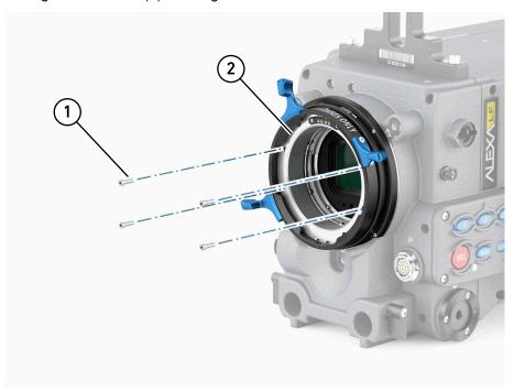
10. Turn the lens lock into Position CLOSED (2) and fasten the other four torx screws hand-tight (1). Check if all screws and the shim fit correctly:
