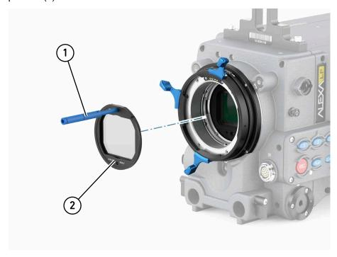
7. Place the next filter onto the bottom ring in the camera's LPL mount. The filter insertion tool has to be in the 12 o'clock position (1).
