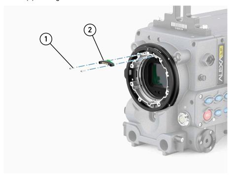
8. Accurately place the LF IFM Shim, with its inscription always facing cameraoutwards (2), onto the LPL mount. The shim's screw holes must line up exactly with the mount's thread holes and the index pin (3):
