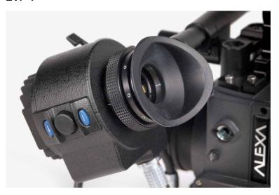
The electronic viewfinder EVF-1 employs a liquid crystal on silicon (LCOS) imaging device with a temperature-stabilized LED light source to provide a bright, accurate view of the sensor image in all operating conditions. Each EVF-1 is calibrated to precisely match the image on the ALEXA's HD-SDI outputs.
