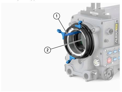
3. Pull the filter (2) from the bottom ring in the camera's LPL mount. If the filter position is held by an LF IFM Empty Filter Frame, remove it likewise.
