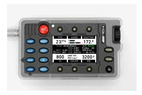
The camera can be remotely controlled with an RCU-4. This device mirrors the controls on the camera's right side. It is connected to the camera's Ethernet port. Power is supplied via the Ethernet cable.
