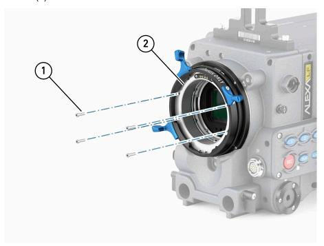
4. Remove the lens lock (1) from the LPL mount. Keep all installed shims (if any) carefully in place (2):
