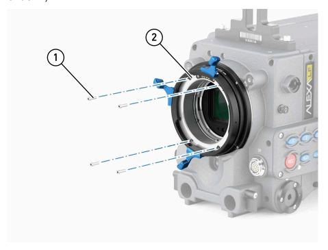
3. Turn the lens lock into position OPEN (2) to unhide and unscrew the other four torx screws (1).
