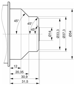
Fig. 8: Allowed lens dimensions with in-camera filters
