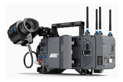
The ALEXA records clips using the recording module on the camera-left side. For every recording medium type, the respective adapter needs to be inserted before a medium can be inserted. The media slot can take SXR Capture Drives with the SXR Capture Drive Adapter and SxS PRO+ cards with the SxS Adapter 2.
