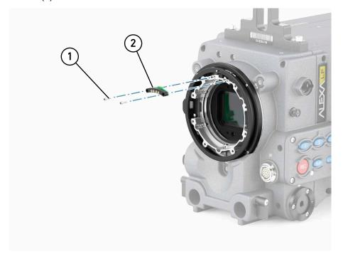
6. Add three 0.1 mm washers (1) on each of the four positioning pins (see detailed section).
