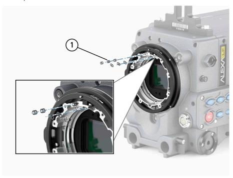
7. Reattach the LDS pin support and MCA print (2) by fastening the two TX6 torx screws (1) hand-tight.
