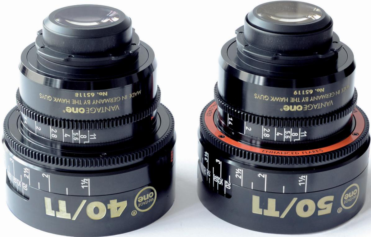
Vantage One lenses will be offered in two versions. The first includes the regular lens coatings, and the second, marked with a distinctive red ring, will incorporate some optical elements with no coating. Leaving some elements uncoated results in additional flaring and lower contrast, qualities that blend very well with the other characteristics of the Vantage One line.
